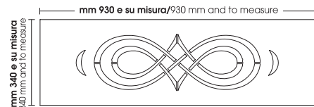
ART. N1/2-09 lamiera spessore mm 4/4 mm thick metal sheet
